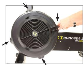
4. Loosen the screw that connects the two ends of the stainless perforated screen, then remove the screen by pulling and unwrapping one end.
